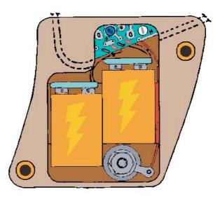
Two volume trim controls are supplied to maintain maximum performance. Both controls have been pre-set at the factory for correct balance in volume between the neck pickup and the bridge pickup.
